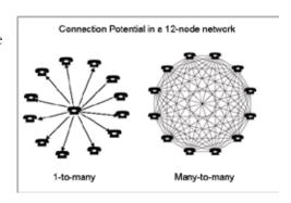
The difference in potential between these two topologies can be seen mathematically and in the diagram at right, which
